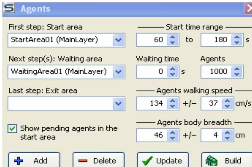
This figure shows the configuration table of SimWalk. This page allows the user to create pedestrians according to their speed and body breadth.
